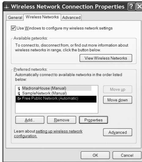
Figure 11-8: Use the Wireless Network Connection Properties window to remove a bogus ad hoc network profile.
