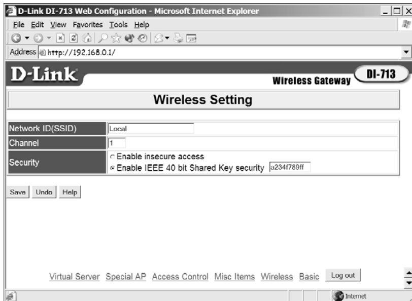
Figure 12-3: The configuration utility for a D-Link access point accepts WEP keys in hex format.
