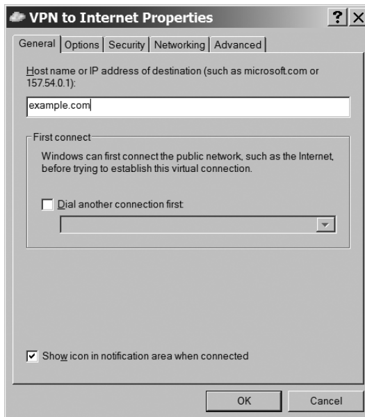
Figure 15-11: The General tab controls the destination of a VPN connection.
