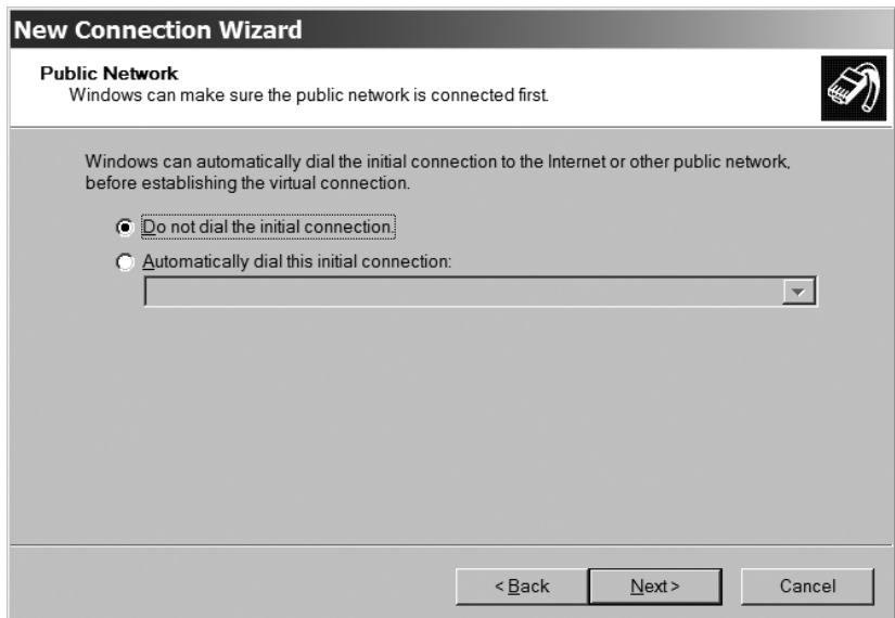
Figure 15-6: In a wireless network, the VPN does not require a dial-up connection.
