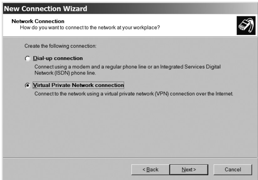
Figure 15-5: Select the Virtual private network connection option to create a VPN connection.
