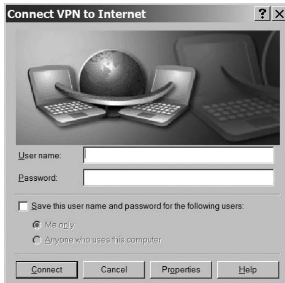
Figure 15-10: Use the Connect VPN to Internet window to configure a VPN in Windows XP.
