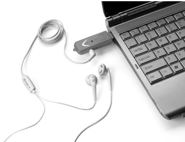
Figure 16-2: Vonage's USB flash drive includes calling software and an earpiece microphone cable.
