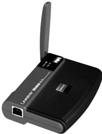
Figure 5-1: This USB Wi-Fi adapter has a permanently attached external antenna.
