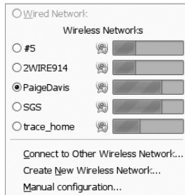
Figure 7-5: NetworkManager is the default Wi-Fi control program for several distributions, including Ubuntu. A KDE version of the program—KNetworkManager—is also available ( http://gnome.org/projects/NetworkManager , http://en.opensuse.org/Projects/KNetworkManager ).
