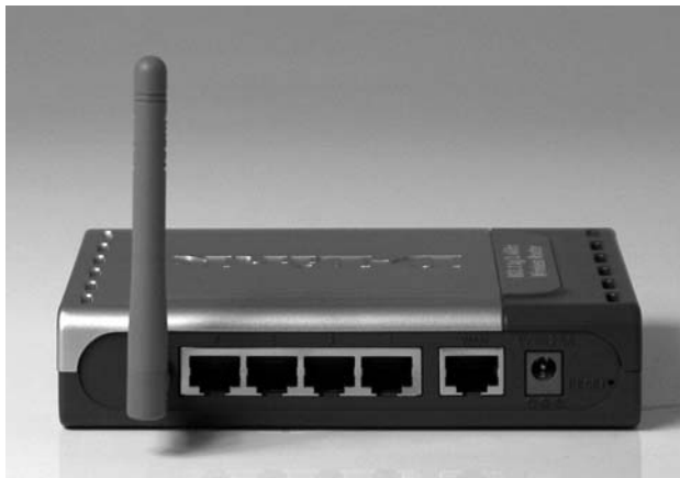
Figure 12-6: The D-Link DI-524 Wireless Broadband Router contains configurable firewall firmware.
