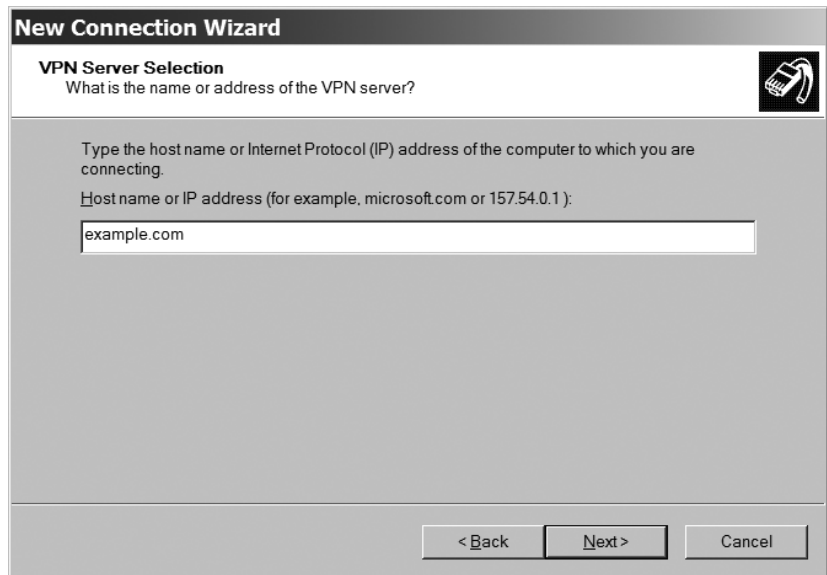
Figure 15-7: The Host Name or IP Address identifies the VPN server at the other end of the wireless link.
