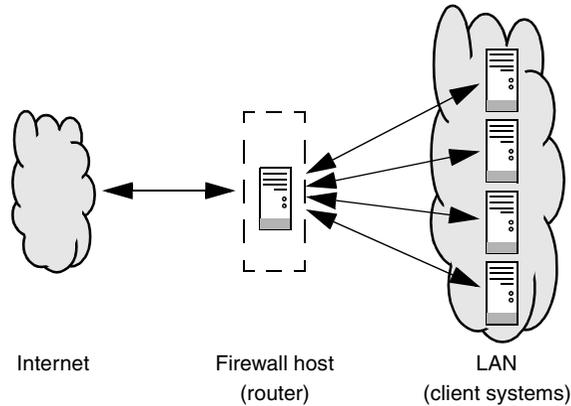
**Figure 26-1** A typical firewall setup
