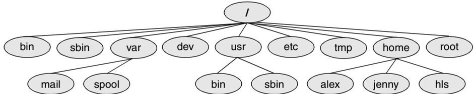
**Figure 6-10** A typical FHS-based Linux filesystem structure
