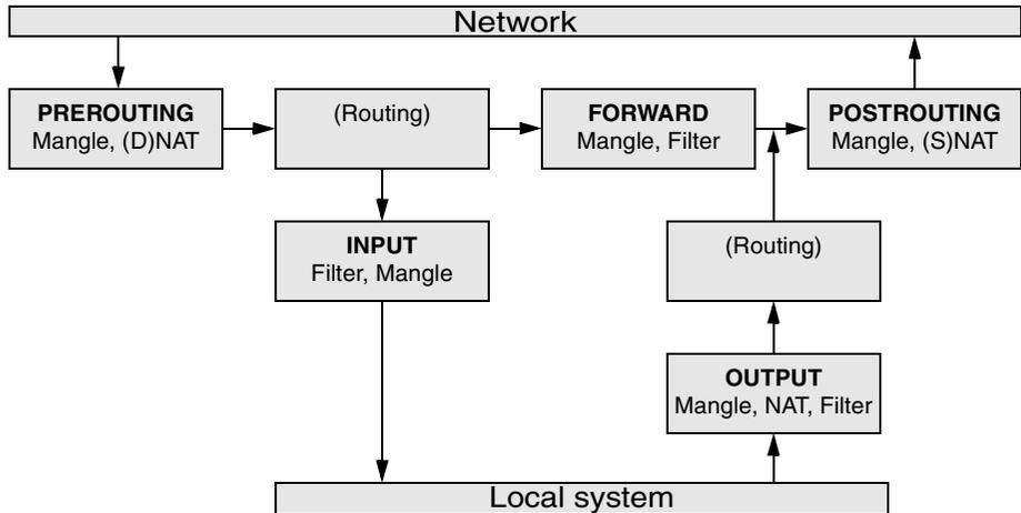
**Figure 26-11** Filtering a packet in the kernel
