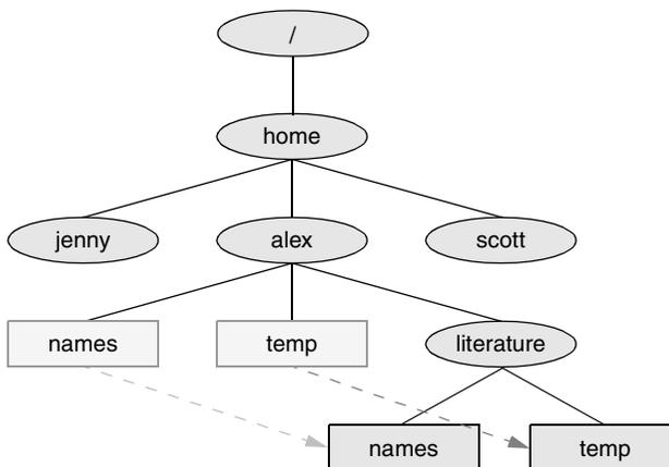
**Figure 6-11** Using `mv` to move `names` and `temp`
