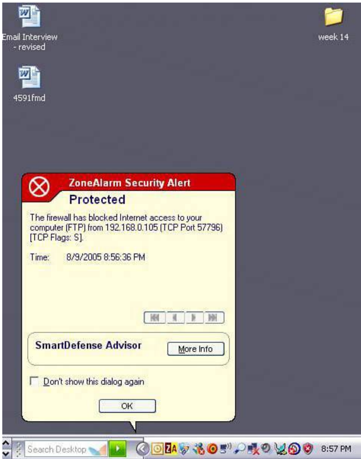
Figure 3.14. Incoming attempts to access your computer are shown in a pop-up alert by ZoneAlarm. This inbound contact is coming from a computer on the same home network.
