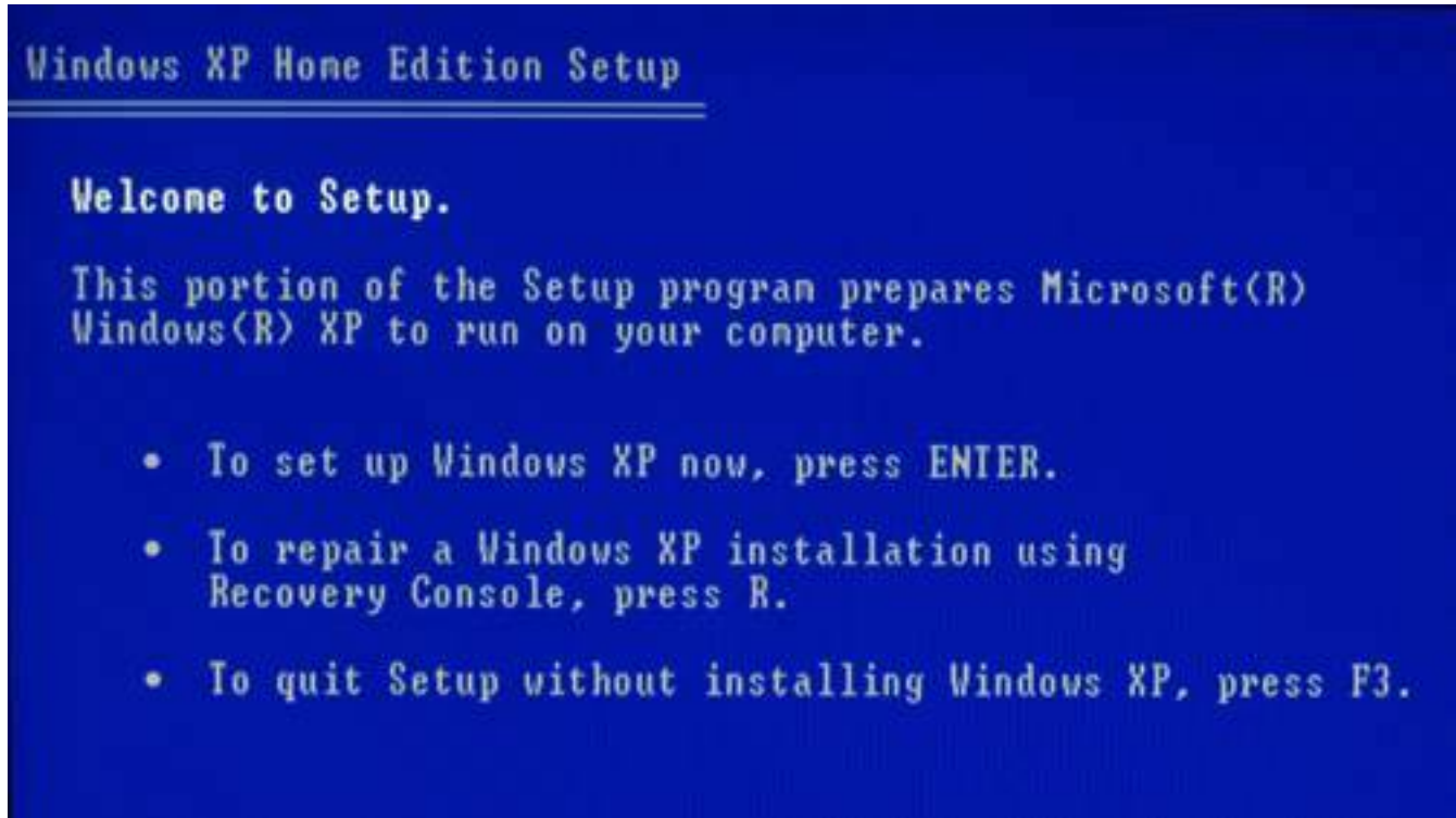
Figure 9.7. When you first boot from the Windows XP CD, you see a blue setup screen like this one.
