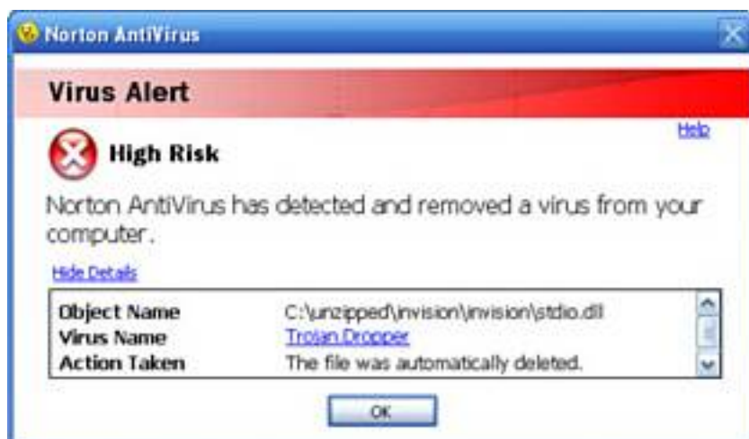
Figure 1.3. This dropper is detected by Norton AntiVirus as it tries to dump a virus or Trojan horse into a Windows XP computer.
