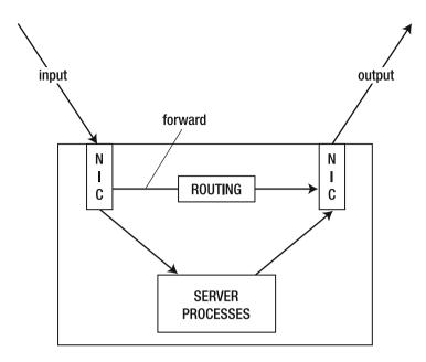
Figure 12-1. Overview of the Use of Netfilter Chains
