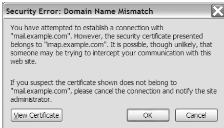
Figure 10-5. Server certificate domain name mismatch failure
