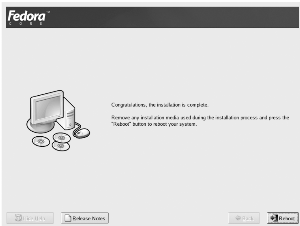
Figure 2-8. When the Fedora Core installer is finished, your installation media will be ejected and your system will be rebooted.
