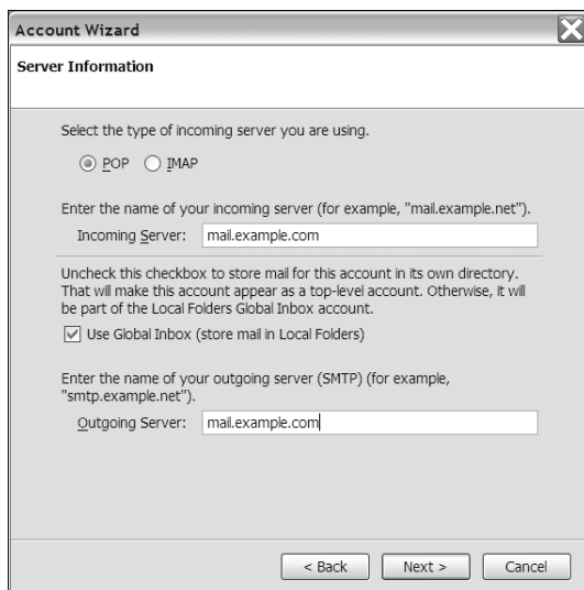
Figure 7-3. Step 3 of the Thunderbird new account setup wizard allows you to add POP or IMAP incoming server and SMTP outgoing server names.
