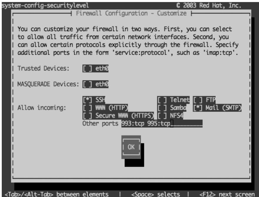
Figure 6-5. Allowing IMAP4S and POP3S through your firewall
