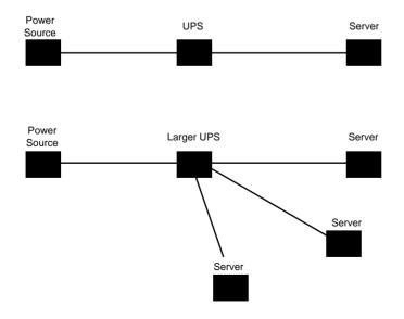
**FIGURE 9.2** A large UPS can service numerous components at once.
