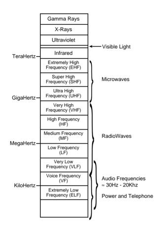
**FIGURE 3.1** The electromagnetic spectrum.
