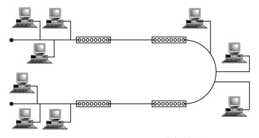
**FIGURE 6.6** 5-4-3 rule: 5 segments connected with 4 hubs, and only 3 segments are populated. <\$Ihubs;types;active>< \$Iactive hubs;signal regeneration><\$Imulti port repeaters><\$Isignal regeneration>
