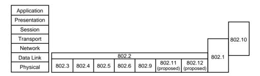
FIGURE 2.14 The relationship between the IEEE 802 standards and the OSI model.
