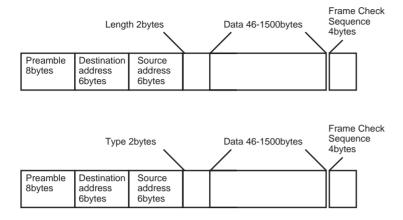
**FIGURE 7.7** An Ethernet II frame type packet.
