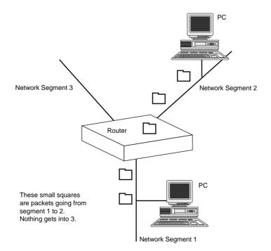
FIGURE 2.9 Routers move packets onto different segments.
