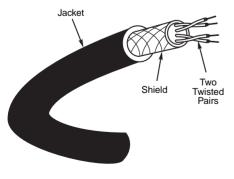
**FIGURE 3.13** A shielded twisted-pair cable.
