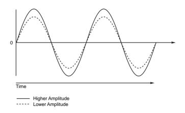
FIGURE 5.4 These two waveforms differ in amplitude.
