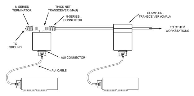
FIGURE 3.10 Connectors and cabling for Thicknet.
