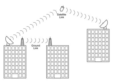
FIGURE 3.21 Terrestrial and satellite microwave links.
