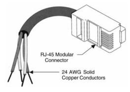
FIGURE 3.17 An RJ-45 connector.
