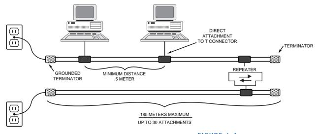
FIGURE 6.4 Using a repeater to extend an Ethernet LAN.
