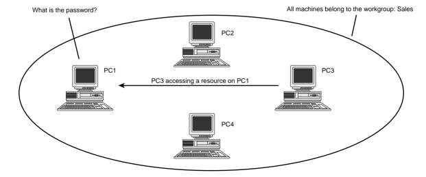
**FIGURE 10.1** A workgroup does not rely on a centralized user account database.
