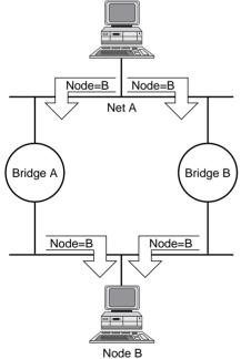
**FIGURE 6.9** A complex network with bridges.
