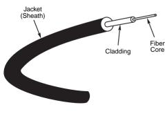
**FIGURE 3.18** A fiber-optic cable.
