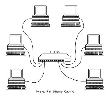
**FIGURE 4.16** A 10BASE-T network wired in a star topology.
