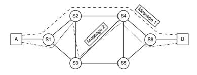
**FIGURE 2.7** Message switching forwards the complete message, one switch at a time.
