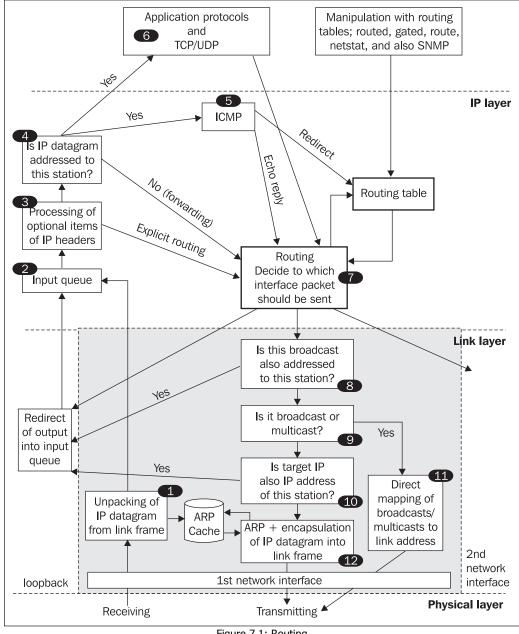
Among other things, Figure 7.1 shows that during the processing of input data, on some occasions, the operating system forwards the information automatically to the output (to the routing process), i.e., application programs do not interfere with the forwarding. These instances include:
