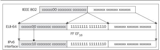
Figure 8.21: Conversion of an IEEE 802 address into an address used in IP version 6
