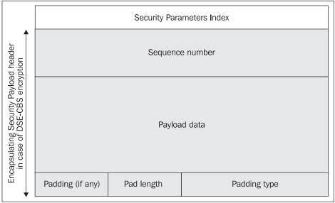
Figure 8.9: Encapsulating Security Payload header
