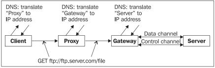
Figure 14.9: A chain of intermediate systems
