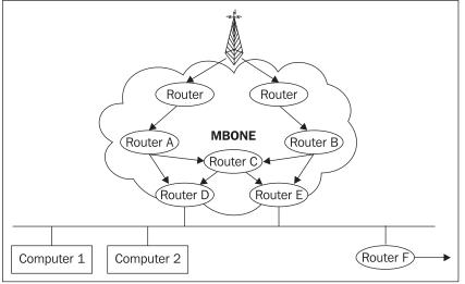
Figure 5.31: Multicasts flooding
