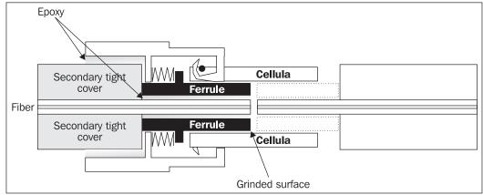
Figure 3.30: The principle of optical connector
