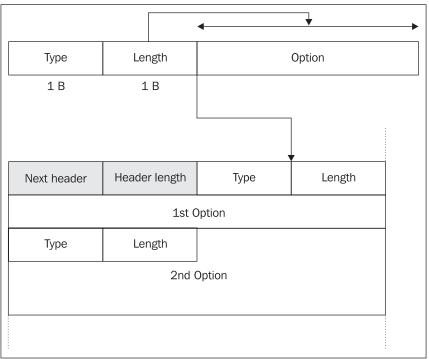
The option (see Figure 8.3) consists of the **Type** field (1 B long), the **Length** field of 1 B and the field containing the **Option** itself.
