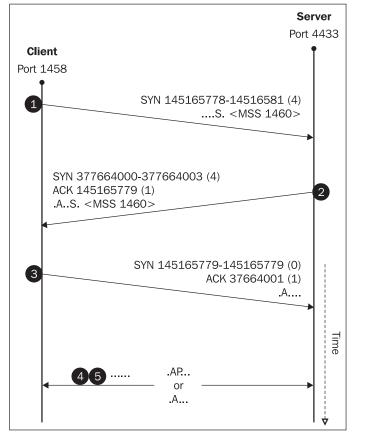
Figure 9.9: Establishing a connection
