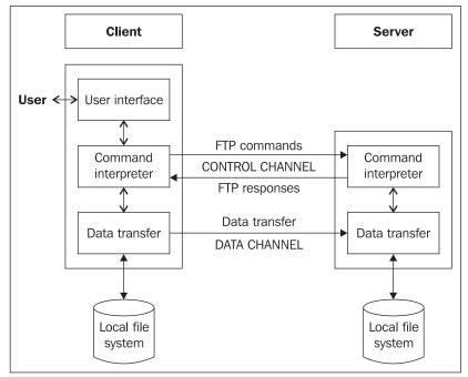
Figure 13.1: The FTP architecture
