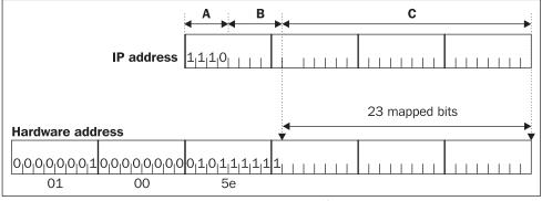
Figure 5.34: Mapping IP multicasts
