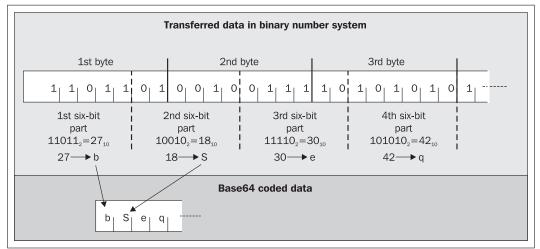
Figure 15.5: Base64 encoding
