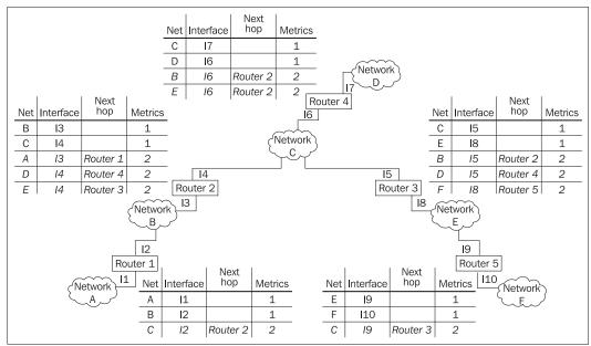
Figure 7.7: The second step of filling routing tables
