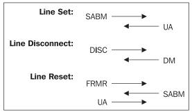
Figure 4.12: Examples of HDLC handshakes
