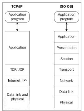
Figure 1.2: Comparison of TCP/IP and ISO OSI network models
