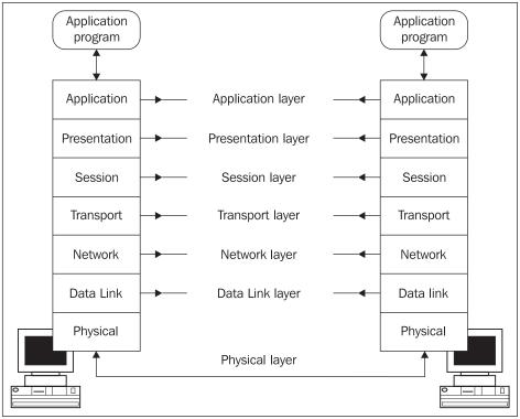
Figure 1.3: Seven-layer architecture of ISO OSI
