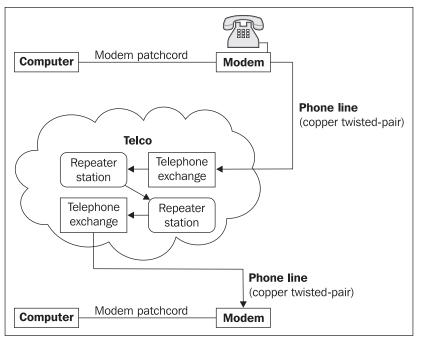
Figure 3.7: Telephone circuit goes through repeater stations and telephone exchanges
