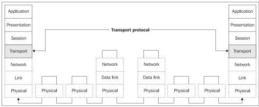
Figure 1.8: Transport layer connection
