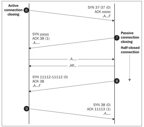
Four TCP segments are required for properly closing a connection. Like the SYN flag in connection establishment, the FIN flag confirms as if it takes up 1 B of data.
