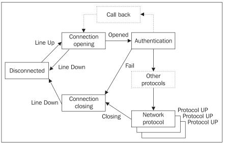
Figure 4.14: Individual link phases in PPP
