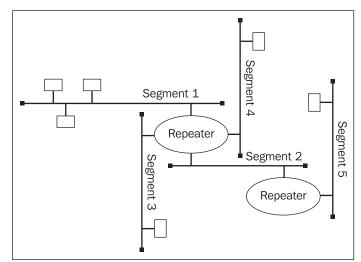
Figure 4.33: LAN consisting of individual segments
