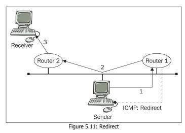
In the figure above, Router 1 receives an IP datagram that needs to be forwarded to another address thorough the same network interface through which the IP datagram came. It forwards the IP datagram, but uses an ICMP redirect packet to instruct the sender to change its own routing table and not to ask for such strange services anymore.
