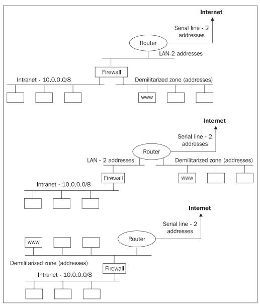
Figure 6.9: The most common firewall connections
