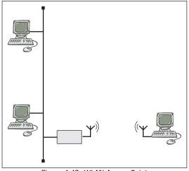
Figure 4.43: WLAN Access Point
