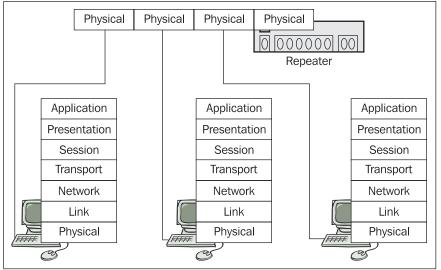
Figure 4.35: Repeater for twisted-pair
