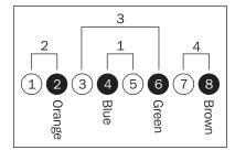
Figure 3.25: EIA 568B-interconnecting individual pairs
