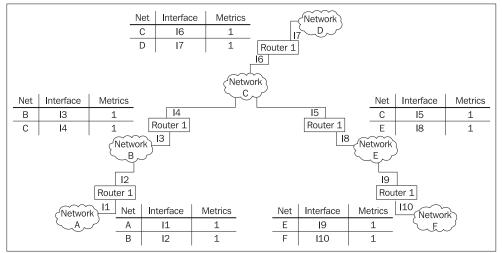
Figure 7.6: The first step of filling routing tables
