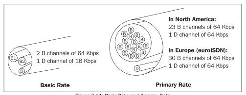
Figure 3.14: Basic Rate and Primary Rate
