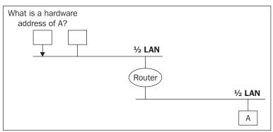
Figure 5.28: LAN separated by a router
