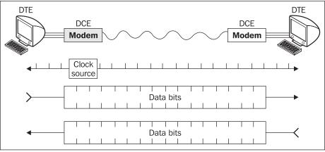
Figure 3.2: Synchronous transport
