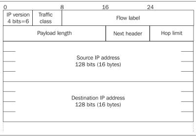
Figure 8.1: Base header of IP version 6 datagram
