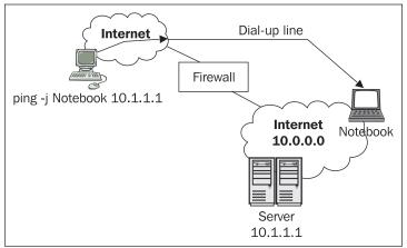
Figure 5.23: Source routing attack
