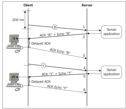
In Figure 9.14, the client using 200 ms delayed the acknowledgements tick.
