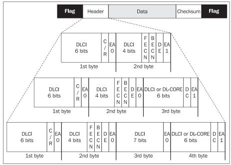
Figure 4.26: Format of Frame Relay frame
