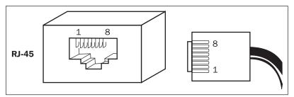
Figure 3.24: The RJ-45 connector
