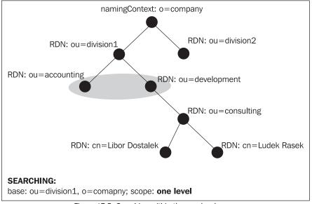
Figure 17.5: Searching within the one-level scope
