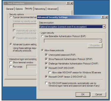
Figure 4.17: Configuration of authentication protocols and encryption in Windows XP
