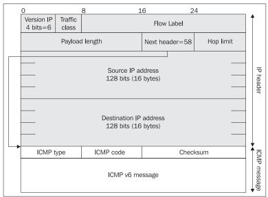
Figure 8.11: ICMP version 6 packet structure
