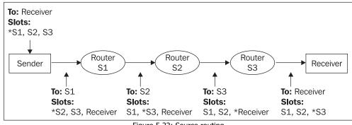
Figure 5.22: Source routing
