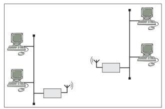
Figure 4.45: Backbone point-to-point connection
