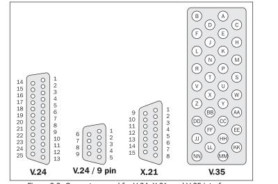
Figure 3.3: Connectors used for V.24, X.21, and V.35 interfaces
