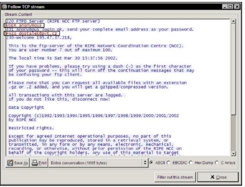
Figure 2.7: TCP connection statements in Ethereal
