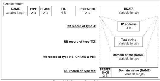
Each RR has the same structure in DNS protocol. The RR structure is shown in the following figure:
