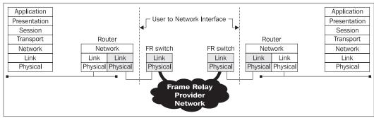
Figure 4.24: Interconnection through the Frame Relay provider
