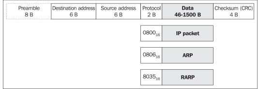
Figure 4.38: Ethernet II frame format
