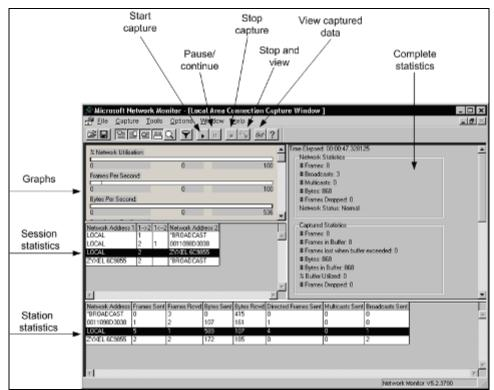
Figure 2.3: Capturing data frames
