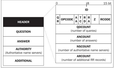
Figure 11.4: DNS Query packet format
