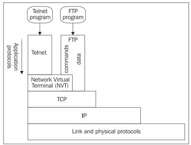
Figure 12.1: Network architecture of the NVT protocol
