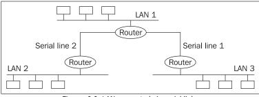
Figure 6.6: LAN connected via serial links
