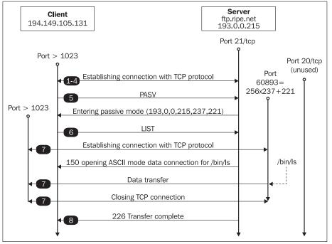
Figure 13.3: FTP passive mode
