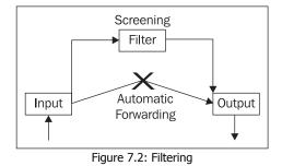
The way screening most often works is that before an IP datagram is forwarded, the whole forwarding procedure is suspended and the decision to forward an IP datagram or not is left to a process (service) running in the background.
