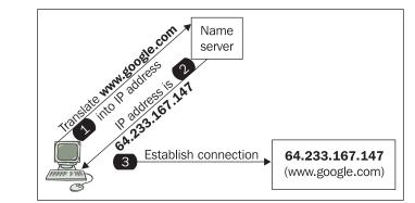
Figure 11.1: It is necessary to translate a name to an IP address before establishing a connection
