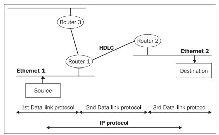
Figure 5.3: Link protocols and IP protocol
