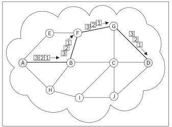
Figure 1.16: Virtual circuit
