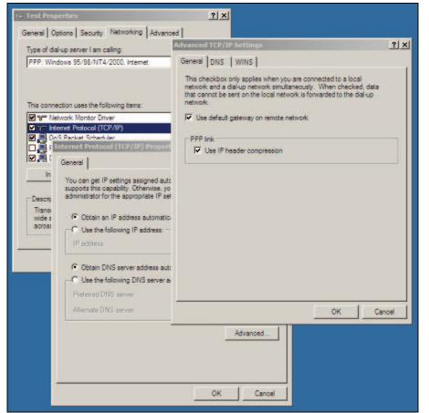
Figure 4.2: IP and TCP header compression can be set when configuring PPP protocol in Windows XP
