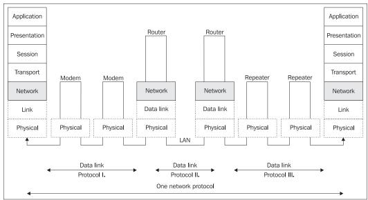
Figure 1.7: Network layer communication
