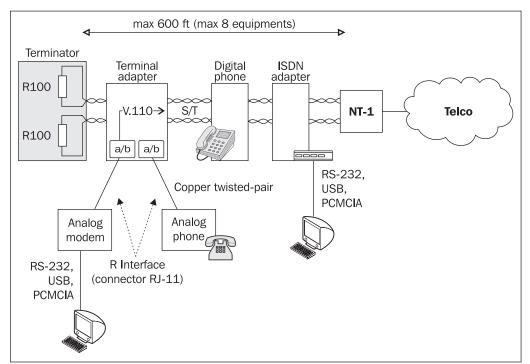
Figure 3.16: Connecting appliances to the S/T interface
