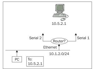
Figure 7.4: Router's dilemma over to which interface should it send the packet.
