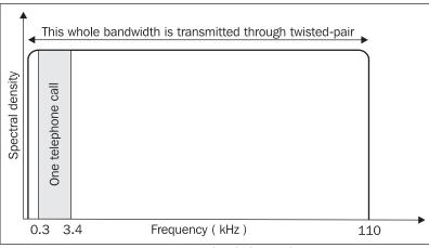
Figure 3.8: Transmission band of twisted-pair wiring
