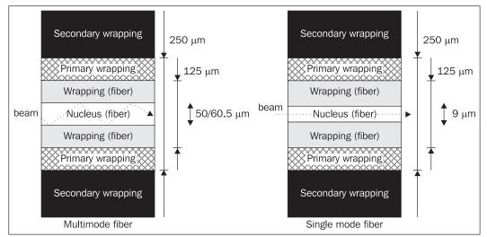
Figure 3.27: Multi- and single-mod fiber
