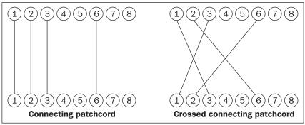
Figure 3.31: TP interconnecting cables
