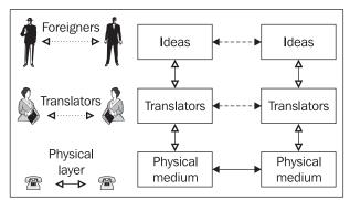
Figure 1.1: Three-layer communication architecture
