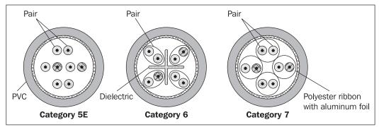
Figure 3.23: Cross section of interconnecting cables
