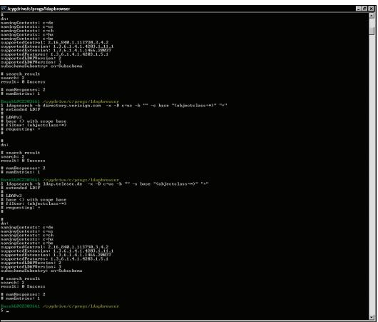
Figure 17.9: An OpenLDAP client command-line utility for LDAP searching
