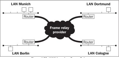
Figure 4.22: WAN based on Frame Relay
