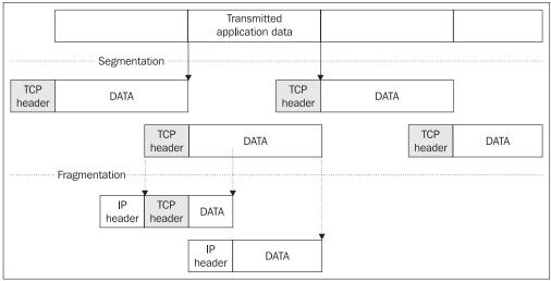
Fragmentation increases overhead, which is why we try to create segments that are not long enough to require fragmentation. Note that the TCP header is transported in the first IP fragment only.
