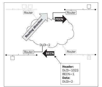
Figure 4.27: Frame Relay Congestion Notification
