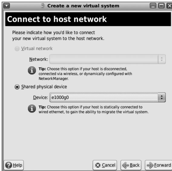
Figure 7-27. Selecting your VM's network device
