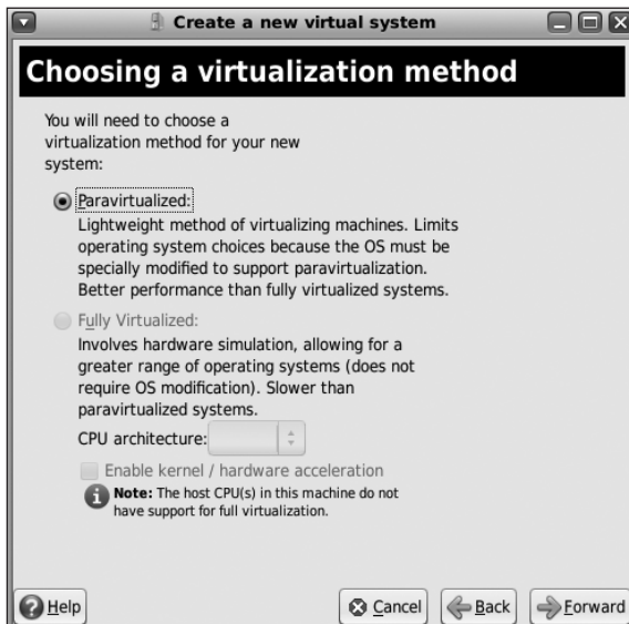
Figure 7-24. Choosing a virtualization method
