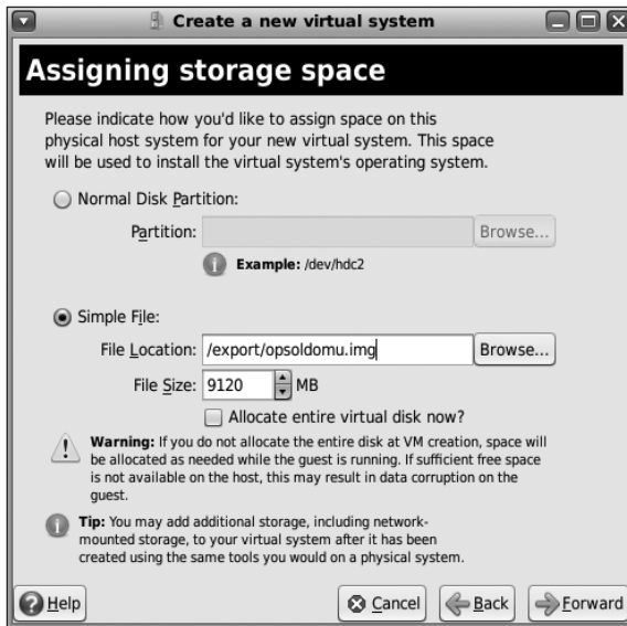
Figure 7-26. Assigning storage space
