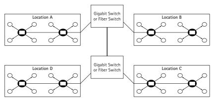
Figure 4-5: A WAN with a gigabit/fiber switched backbone
