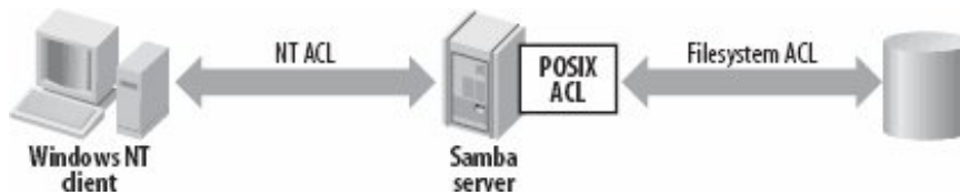
Figure 6-3. Mapping from Windows security descriptors to Unix filesystem ACLs
