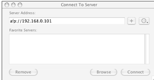
Figure 26-2: In Mac OS X, see Samba and AppleTalk shares from the Connect To Server window.
