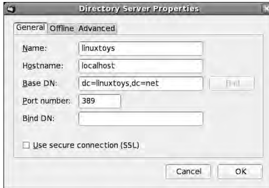
Figure 22-1: Enter information about your LDAP directory server to search for addresses from Thunderbird.
