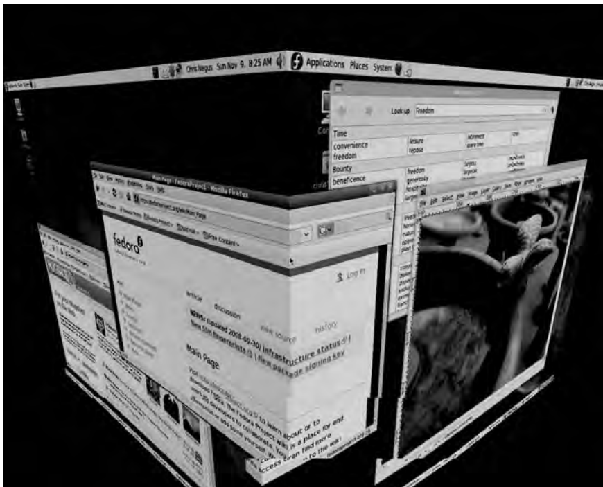
Figure 3-23: With AIGLX enabled for the Compiz window manager, windows wobble as you move them around on the desktop and workspaces spin on a cube.
