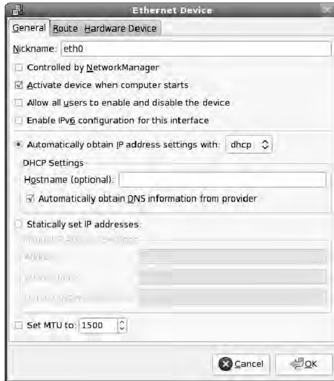
Figure 15-10: Configure your eth0 interface using the Ethernet Device window.
