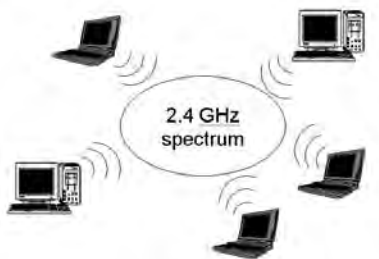
Figure 15-6: Wireless LANs can communicate as peers by broadcasting data.
