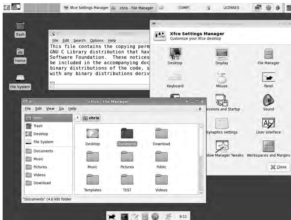
Figure 3-24: Xfce offers a lightweight desktop environment, with applications designed to launch and run quickly.
