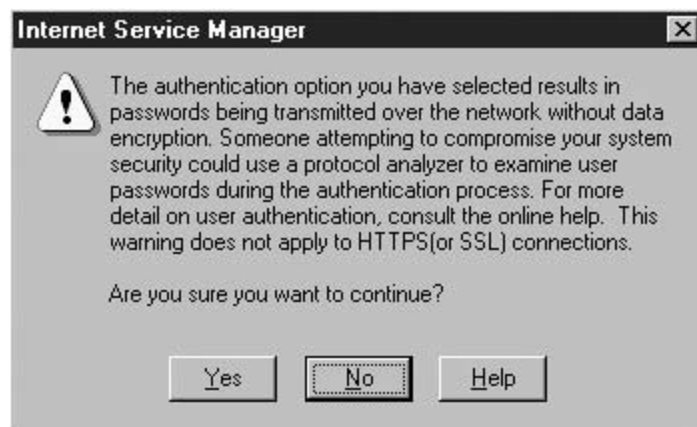
Figure 5-6. Password Vulnerability Warning
