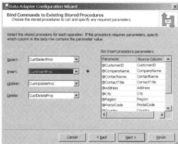
Figure 8.11: The screen from Figure 8.10 after stored procedures have been selected. The mapping of data columns to stored procedure parameters is shown in the grid on the right.
