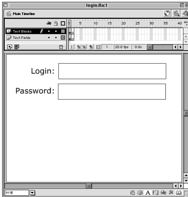
Figure 21-3: Here we have four text areas: two Static Text blocks on the left, and two Input Text fields on the right. The Static Text cannot be altered and/or “read” by ActionScript.
