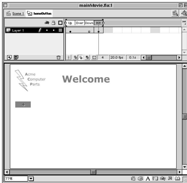
Figure 13-12: The Hit state defines the “active” area of the Button instance in the movie. If the user’s mouse pointer enters this area, then the Over frame of the Button will be displayed.
