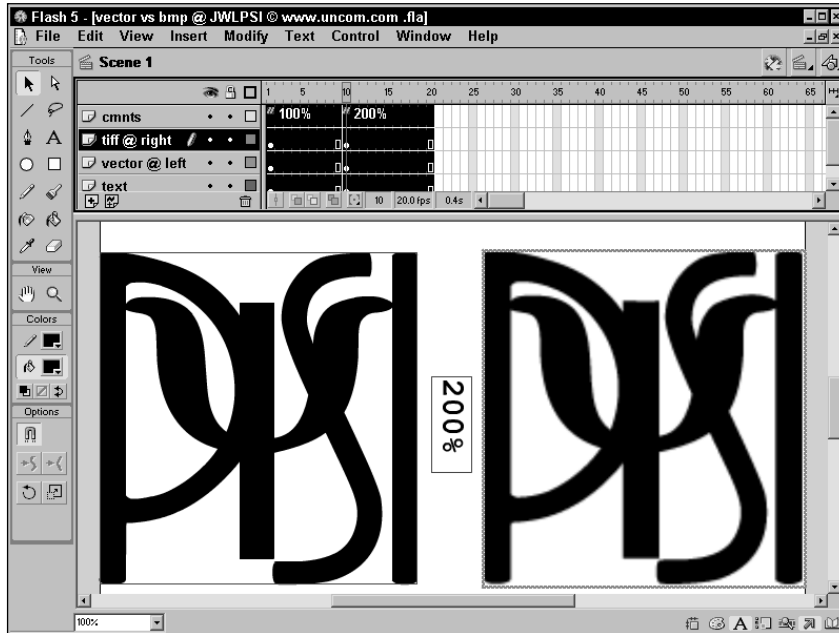
Figure 12-2: Here's JWL's logo again. Now compare the scaled vector graphic on the left to the scaled bitmap image on the right – the vector is clearly superior.
