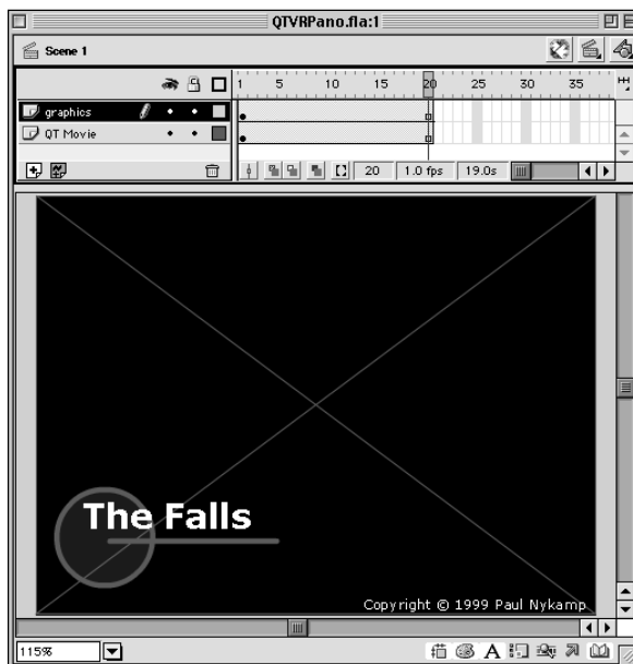
Figure 34-11: If your Flash movie plays beyond the length of an imported QTVR panorama or object movie, it disappears from the stage and is replaced with a struck-through box.
