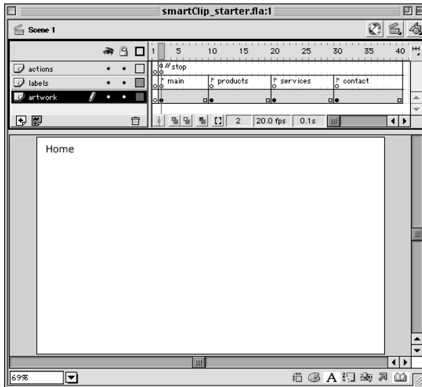
Figure 23-2: The Main Timeline should demonstrate the layout of the Flash movie sections.
