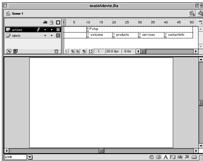
Figure 13-4: Unlike labels, frame comments can not be used in ActionScript. Comments can provide quick visual references for ActionScript code.
