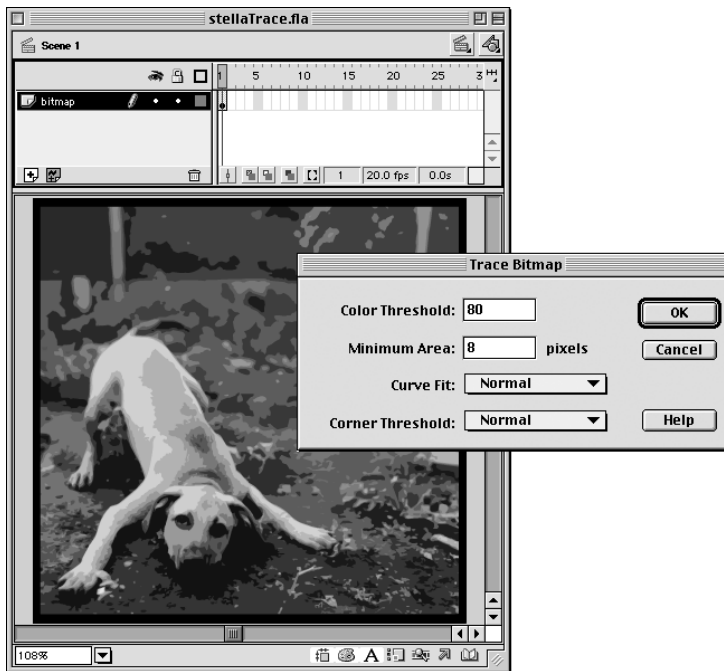
Figure 31-14: The Trace Bitmap command can be used to convert bitmap images into vector Flash artwork. Higher Minimum Area and Color Threshold values reduce the complexity of the resulting Flash artwork, which means smaller Flash movies.
