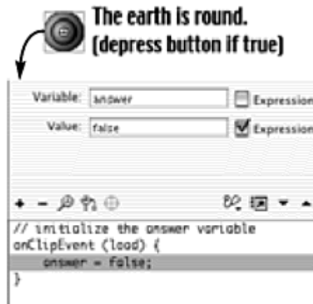
Figure 9.51. The radio-button movie clip initializes the answer variable to the Boolean value false
