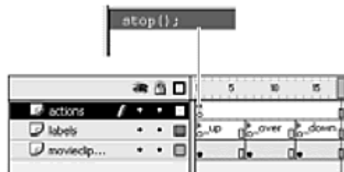
Figure 4.57. Add a stop action to the first frame to prevent the movie clip from playing automatically.
