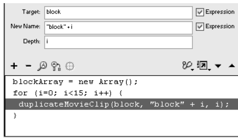
Figure 11.42. The movie clip called block on the Stage is duplicated and automatically given a new name based on the loop variable i .
