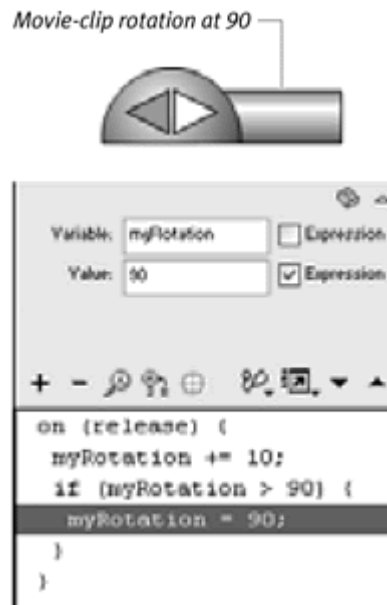
Figure 9.46. The cannon turret can't rotate past 90 degrees, because the if statement won't allow the variable myRotation to increase beyond 90.
