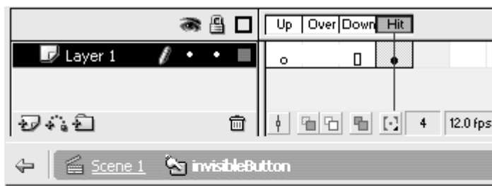
Figure 4.14. An invisible-button symbol. The rectangle in the H i t keyframe defines the active area of the button.
