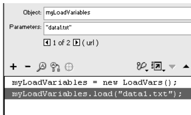
Figure 9.21. The load() method loads the data.txt file from the same directory as the Flash movie and puts the variables in the myLoadVariables object.
