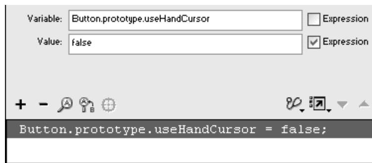
Figure 11.94. All button instances will inherit the property useHandCursor = false , so the hand icon will not appear.
