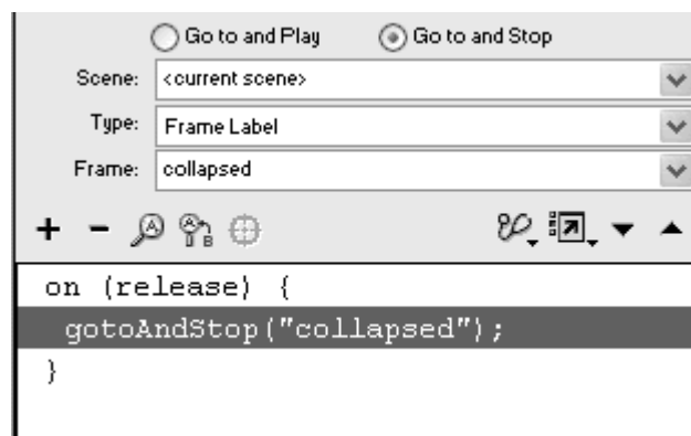
Figure 4.33. This button sends the Flash playhead to the frame labeled collapsed and stops there.
