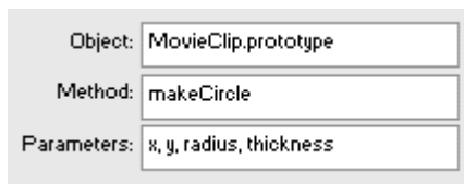
Figure 11.91. The makeCircle() method is assigned to the MovieClip class. This method passes four parameters: x , y , radius , and thickness .
