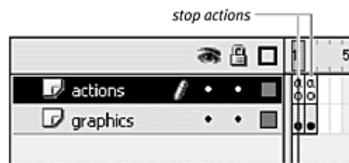
Figure 5.44. The radio-button movie clip contains a stop action in both keyframes and two different states that toggle.
