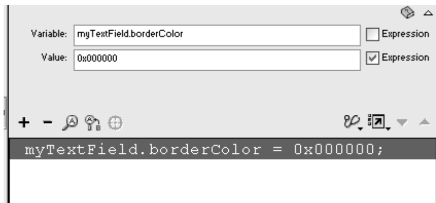
Figure 3.53. The borderColor property takes a hex number as its value. The final statement makes the border color of the text box called myTextField black.
