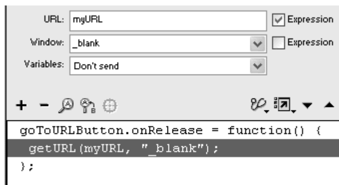
Figure 10.3. The actions assigned to the button called goToURLButton load the URL with the variable myURL in a new browser window.
