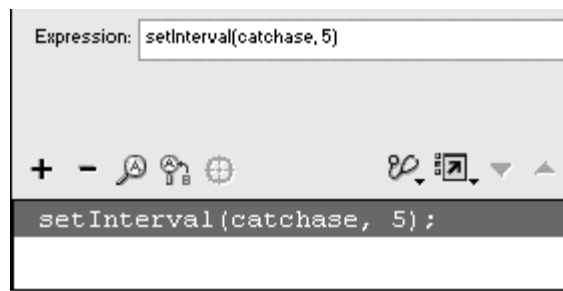
Figure 7.110. The action setInterval , like the event handler onEnterFrame , is a good way to execute ActionScript statements continuously.
