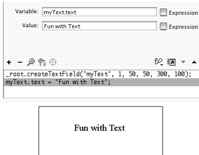
Figure 10.50. The contents of the text property of myText appear on the Stage. The default format for a dynamically created text field is black 12-point Times New Roman (Windows) or Times (Mac).
