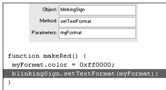
Figure 10.66. A portion of the Script pane shows the function called makeRed , which changes the text field called blinkingSign to a red Forte font.
