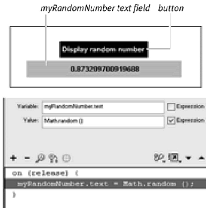
Figure 11.28. A random number between 0 and 1 is displayed in the text field called myRandomNumber when the button is clicked.
