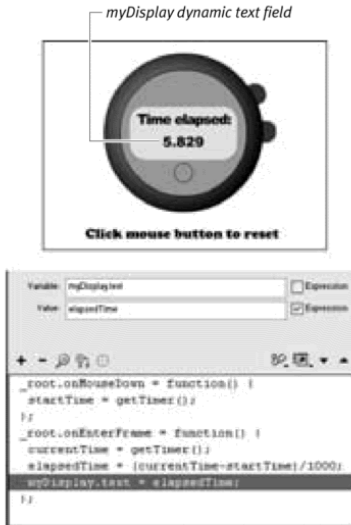
Figure 11.65. The value of elapsedTime is displayed in the text field called myDisplay (top).
