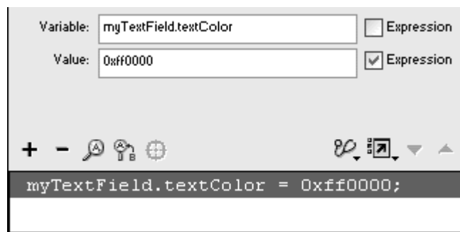
Figure 10.29. The textColor property of the text field called myTextField is set to red.
