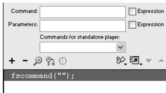
Figure 6.70. fscommand options for projectors appear in the pull-down menu at the bottom of the Parameters area.
