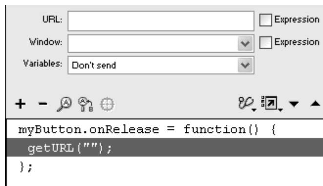
Figure 6.1. The getURL action has parameters for a URL, window name, and methods of sending variables to CGI scripts.
