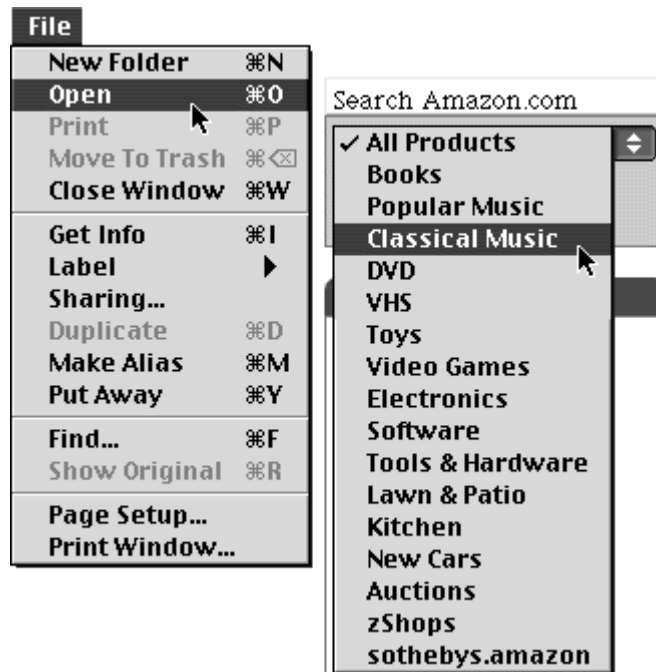
Figure 4.28. Typical pull-down menus: the Mac OS File menu (left) and a Web menu from Netscape Navigator (right).
