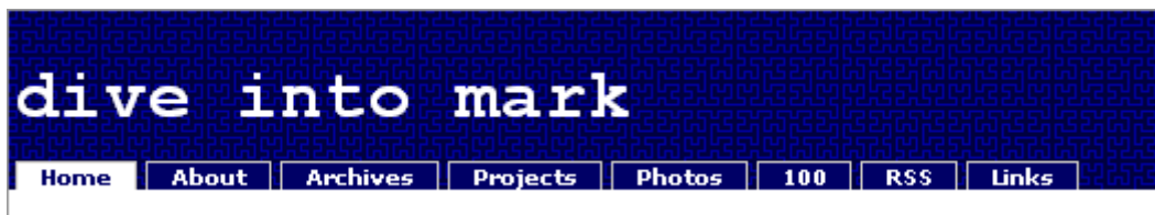
Figure 5 - Mark Pilgrim's site (divintomark.org) sports this tabbed navigation, which uses an unordered list and CSS to style it.
