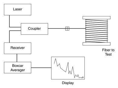
Figure 17-10 An OTDR block diagram.
