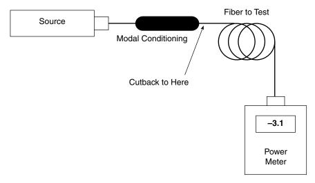
Figure 17-8 Fiber attenuation by cutback method.
