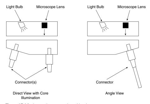
**Figure 17-14** Inspecting connection with microscope.
