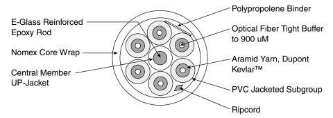
Figure 4-5 Tightpack cable shown in cross-section.
