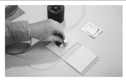
Figure 6-6 A polishing puck holds the connector properly for polishing.
