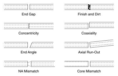
Figure 6-1 Connector loss factors.
