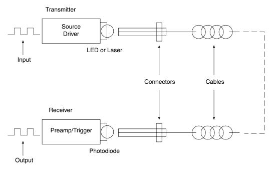
**Figure 17-18** Typical fiber optic link.
