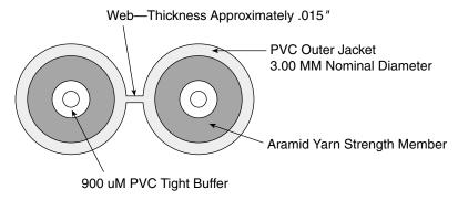
Figure 4-4 Zipcord cable shown in cross-section.
