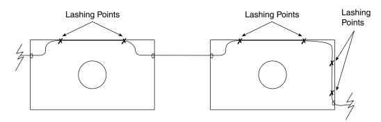
Figure 15-7 Racking cable in manholes.
