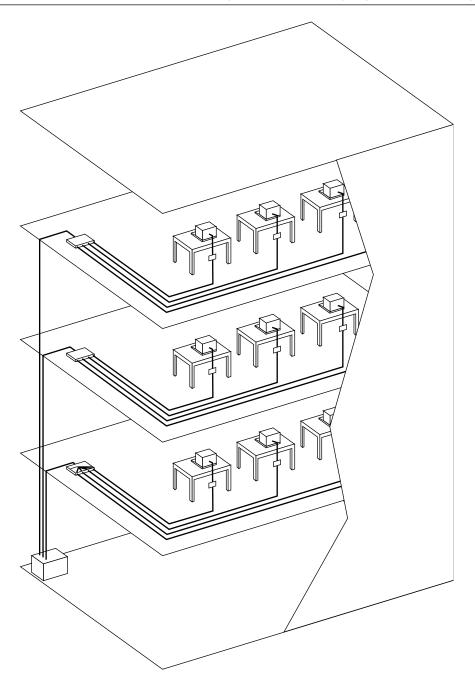
**Figure 7-2** "Homerun" or centralized fiber cabling system.
