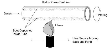
Figure 2-5 Modified chemical vapor deposition (MCVD).
