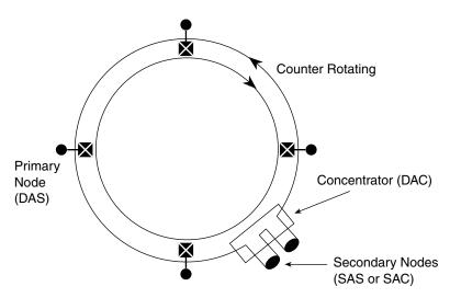
**Figure 3-3** Fiber distributed data interface (FDDI).
