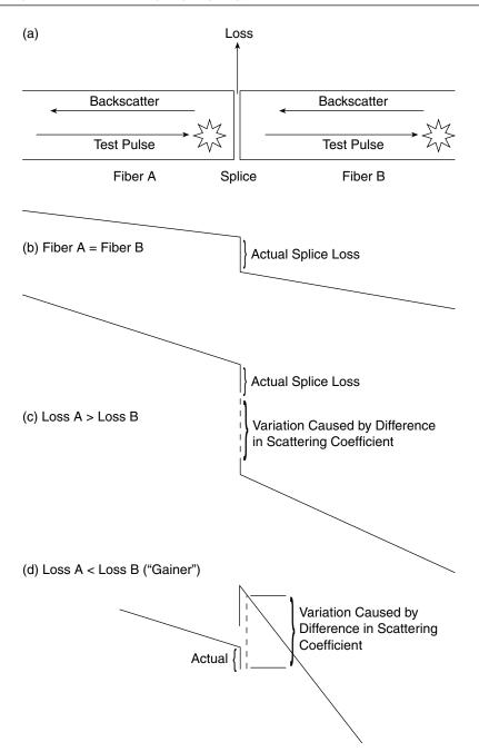
Figure 17-12 OTDR loss measurement uncertainty.
