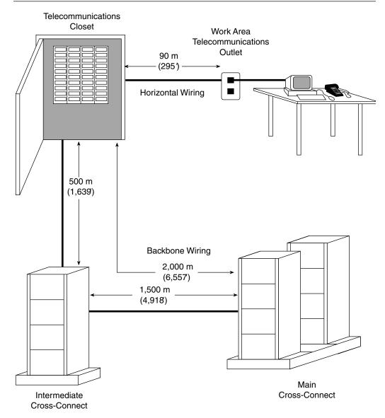
Figure 7-1 Backbone cabling.
