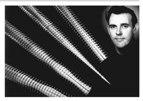
**Figure 1-10** George Hockham with the metal waveguides he made to model waveguide transmission in fibers. Courtesy BNR Europe
