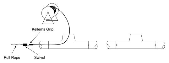
**Figure 15-3** The first half of a multistage pull.
