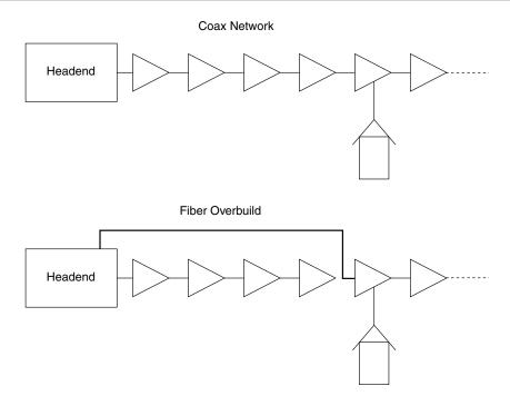
Figure 3-2 CATV architectures before and after fiber overbuild.
