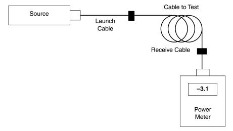
Figure 17-16 Double-ended cable loss test.
