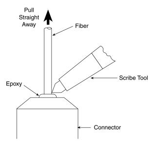
**Figure 6-5** The fiber is epoxied into the connector body, then scribed and broken off just above the connector face before polishing.
