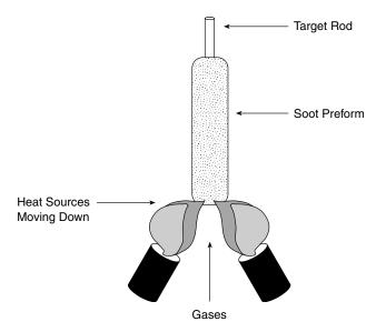
Figure 2-7 Vapor axial deposition (VAD).
