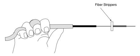
Figure 15-8 Holding cable for stripping fiber.
