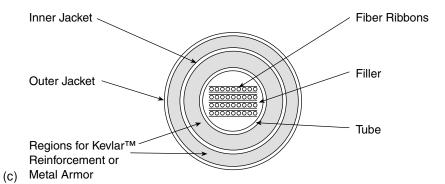
**Figure 4-1** (a) Tight buffered fiber optic cable. (b) Loose-tube fiber optic cable. (c) Ribbon fiber optic cable.
