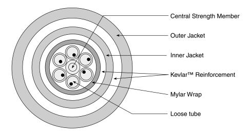
**Figure 4-7** Loose-tube cable shown in cross-section.
