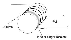
Figure 15-6 Using a mandrel for pulling cable.
