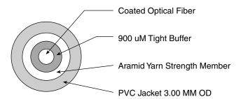
**Figure 4-3** Simplex cable shown in cross-section.
