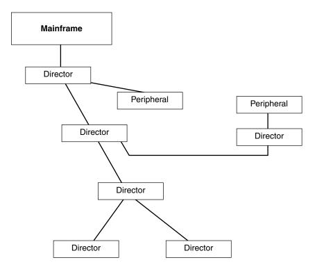
**Figure 3-4** Enterprise system connection (ESCON) architecture.
