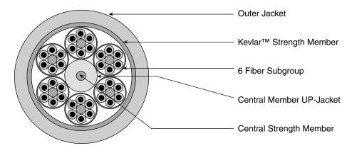
**Figure 4-6** Breakout cable shown in cross-section.
