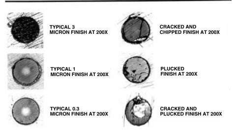
**Figure 17-7** Connector faults are easily seen through a microscope. Courtesy Buehler LTD
