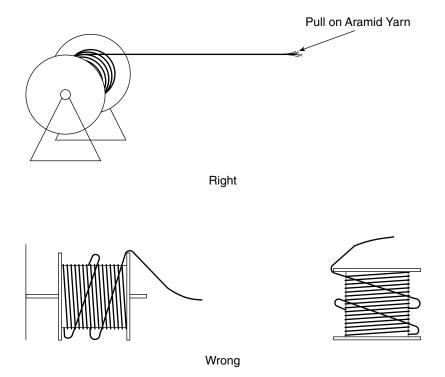
**Figure 15-2** Despooling fiber optic cable.
