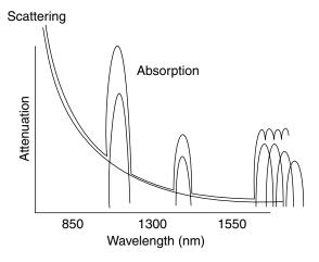
Figure 2-10 Fiber loss mechanisms.
