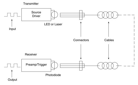
Figure 2-1 A typical fiber optic data link.
