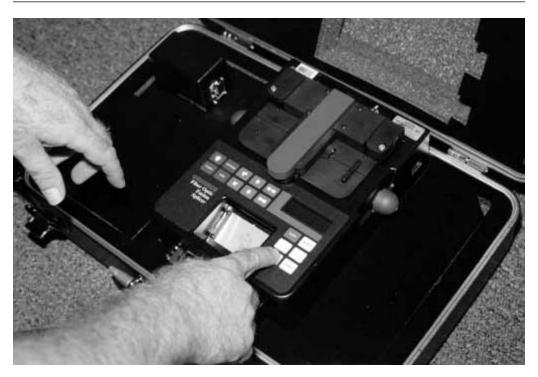
Figure 6-9 Fusion splicer.
