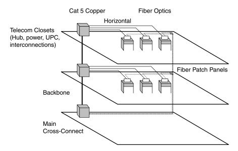
**Figure 3-5** Fiber and copper use different network architectures.
