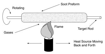
Figure 2-6 Outside vapor deposition (OVD).
