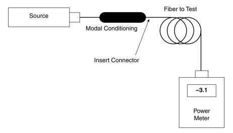
Figure 17-13 Connector insertion loss test.
