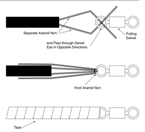
Figure 15-5 Attaching pulling swivel to cable strength member.
