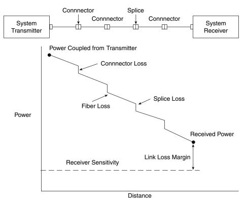
**Figure 10-1** Fiber optic link loss budget.
