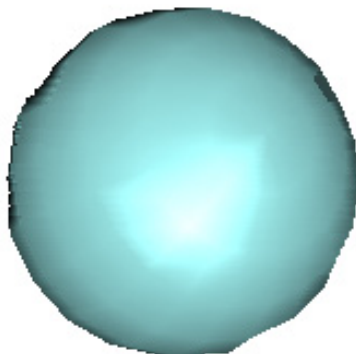
Figure 6. Sphere Rendered Using Gouraud's Smooth-Shading Method
