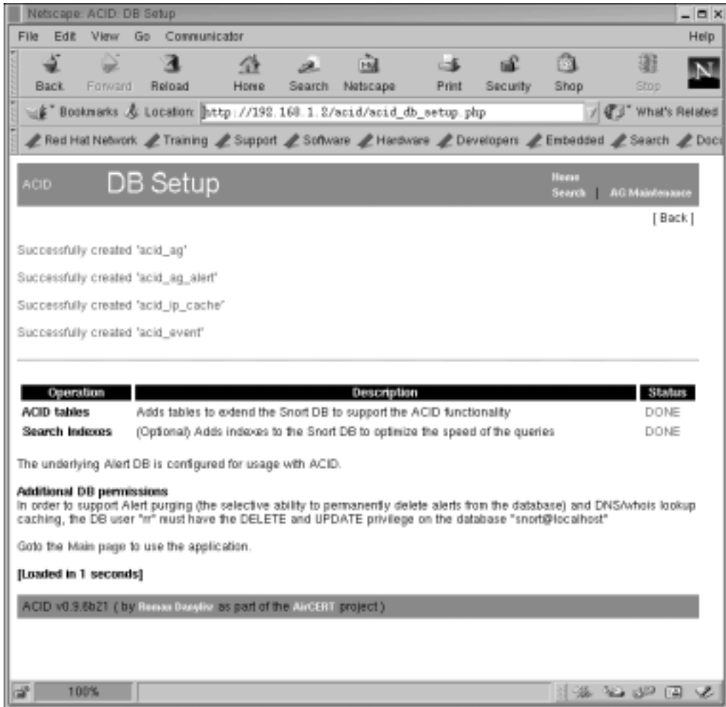
Figure 6-3 The result of creating additional tables in the Snort database to support ACID.
