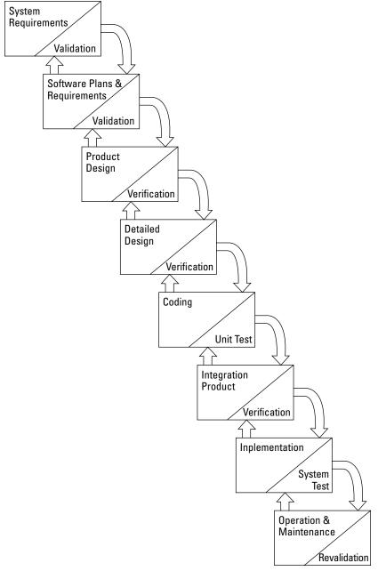
Figure 7-3: A modified Waterfall model incorporating V&V.
