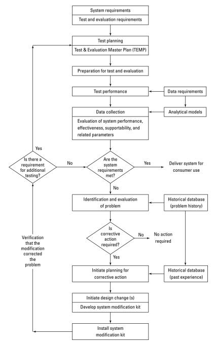
**Figure 13-4:** Security system test and evaluation corrective-action loop. (Source: B. Blanchard, Systems Engineering Management, Third Edition, Wiley Publishing, Inc., 2004. Used by permission.)
