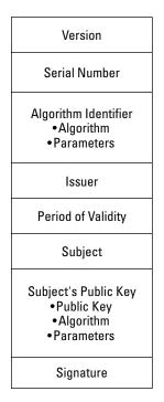
Figure 4-15: The CCITT-ITU/ ISO X.509 certificate format.
