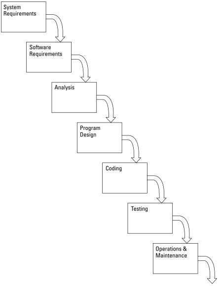
Figure 7-1: A simplistic software development model.
