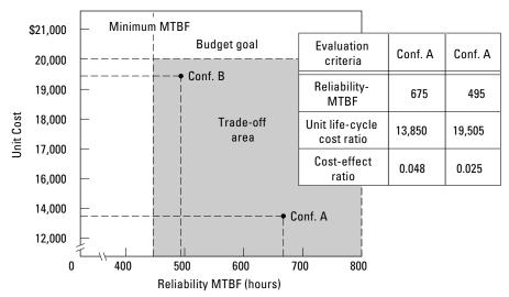
Figure E-18: Reliability versus unit life cycle cost.
