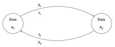
Figure 5-9: State transitions defined by the function f with an input X.
