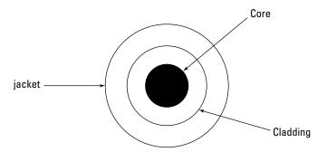
Figure 3-7: Fiber-optic cable cross-section.
