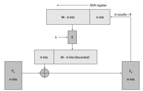
Figure 4-12: DES Cipher Feedback operation.
