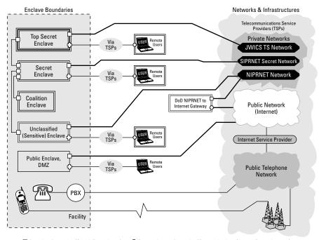
□ Boundary Protection (Guard, Firewall, etc.) Gremote Access Protection (Communications Servers, Encryption, etc.) Figure 11-17: A typical DII site (from IATF document, Release 3.1, September 2002).
