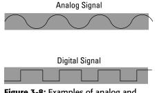
Figure 3-8: Examples of analog and digital signals.
