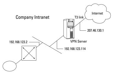
Figure 3-27: A common VPN configuration.
