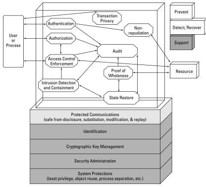
Figure 11-20: Technical security controls (from NIST SP 800-30).
