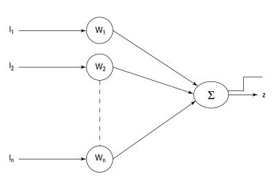
Figure 7-7: A single-layer artificial neural network.
