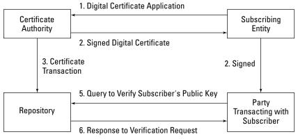
Figure 4-14: A transaction with digital certificates.
