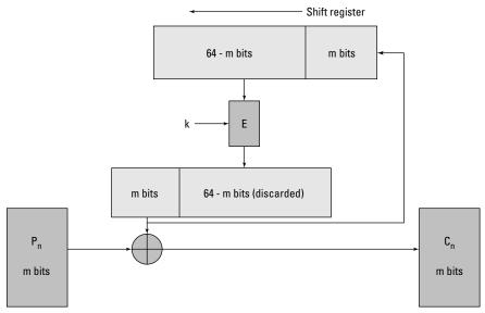
Figure 4-13: DES Output Feedback operation.
