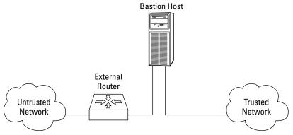
Figure 3-22: A screened-host firewall.
