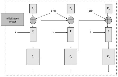
Figure 4-11: Cipher Block Chaining (CBC).
