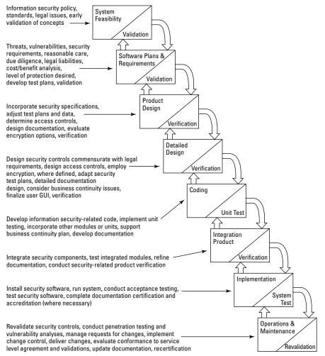
Figure 7-5: Security life cycle components.
