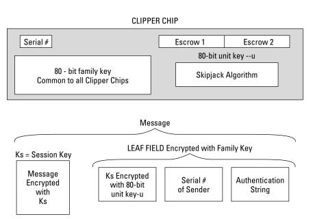
Figure 4-17: A Clipper Chip block diagram.
