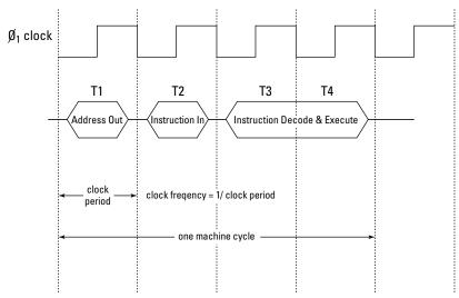
Figure 5-3: A typical machine cycle.
