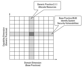
**Figure 13-1:** The capability and domain dimensions of the SSE-CMM.
