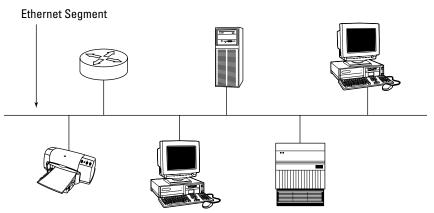
Figure 3-5: Ethernet network segment.
