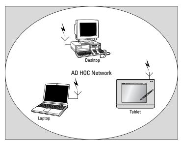
Figure 3-35: WLAN ad hoc mode.
