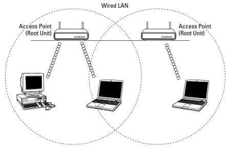
Figure 3-36: Infrastructure Mode 802.11b WLAN.
