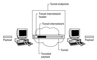
Figure 3-31: VPN tunnel and payload.
