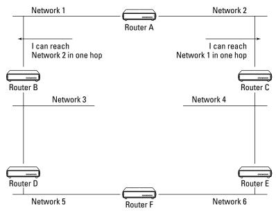
Figure 3-18: Distance vector routing.
