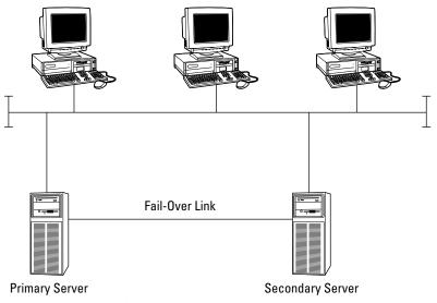
Figure 3-33: Redundant servers.
