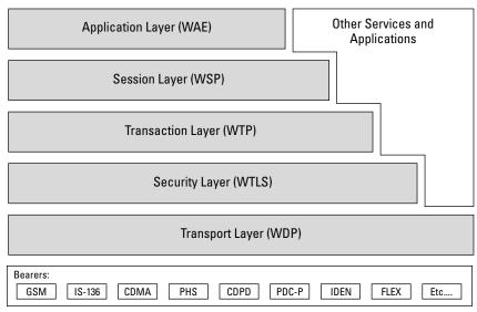
Figure 3-37: The Wireless Application Protocol.
