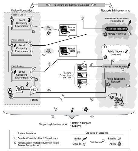
**Figure 11-14**: Relationships of the classes of attacks to computing environment enclaves (from IATF document, Release 3.1, September 2002).
